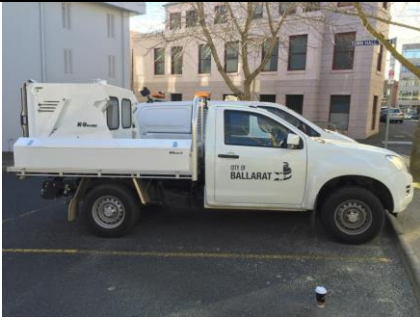
Image 1 Utility with hydraulic animal enclosure
