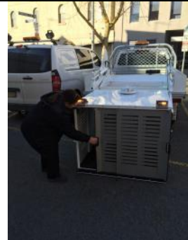
Image 3 Posture assumed to open hydraulic animal enclosure
